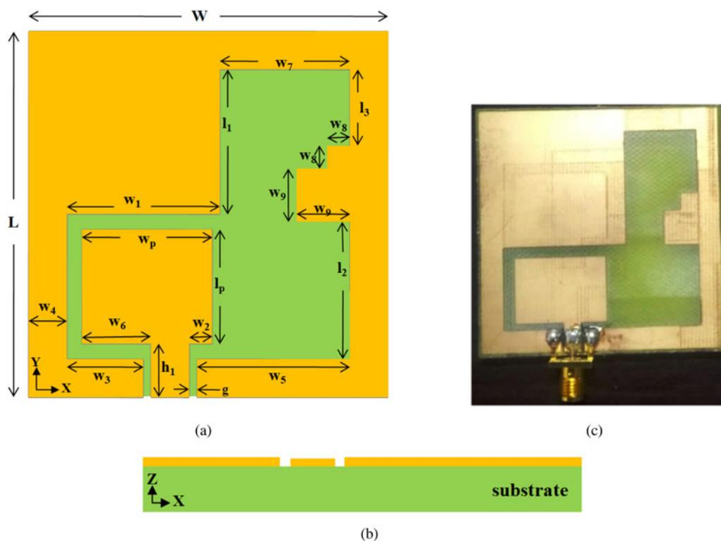
Fig. 1. Geometry of the proposed antenna: (a) top view, (b) side view, (c) fabricated prototype.
