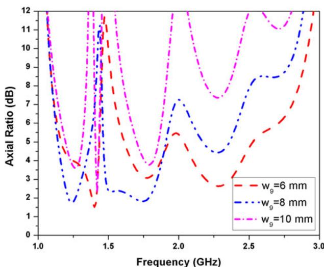
Fig. 10. Simulated axial ratio with different values of  $w_9$ .
