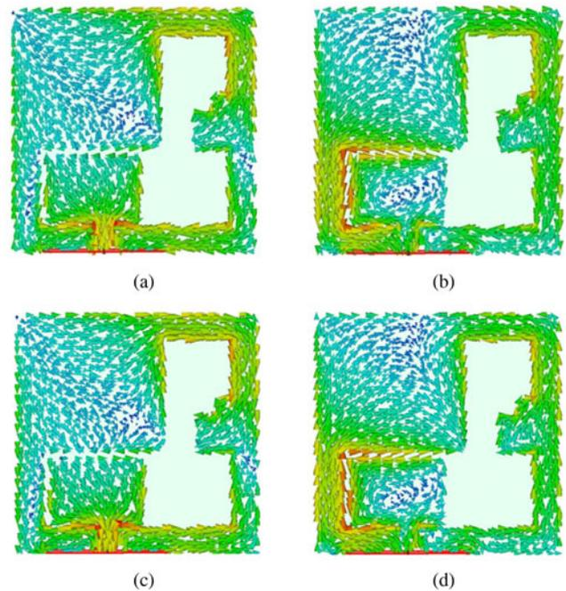
Fig. 7. Current distribution of the proposed antenna at 1.58 GHz: (a)  $\omega t = 0^\circ$ , (b)  $\omega t = 90^\circ$ , (c)  $\omega t = 180^\circ$ , (d)  $\omega t = 270^\circ$ .
