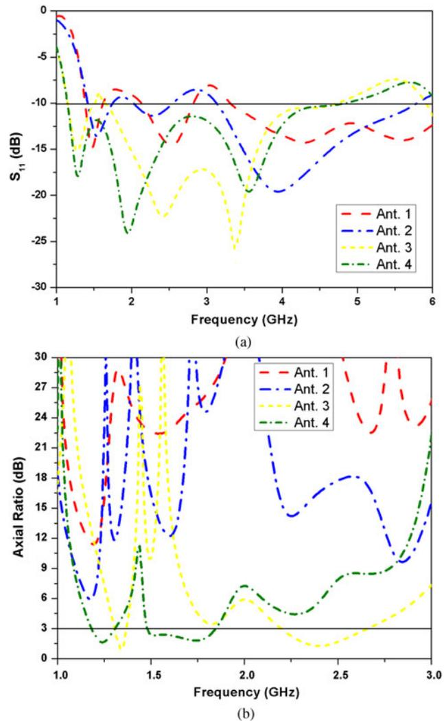
**Fig. 3.** Performance comparison of antenna designing steps: (a) magnitude of  $S_{11}$ , (b) axial ratio.
