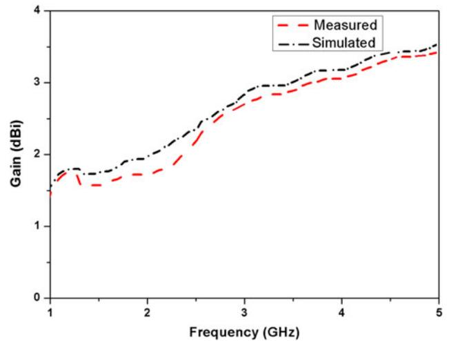
Fig. 6. Simulated and measured gain of the proposed antenna.
