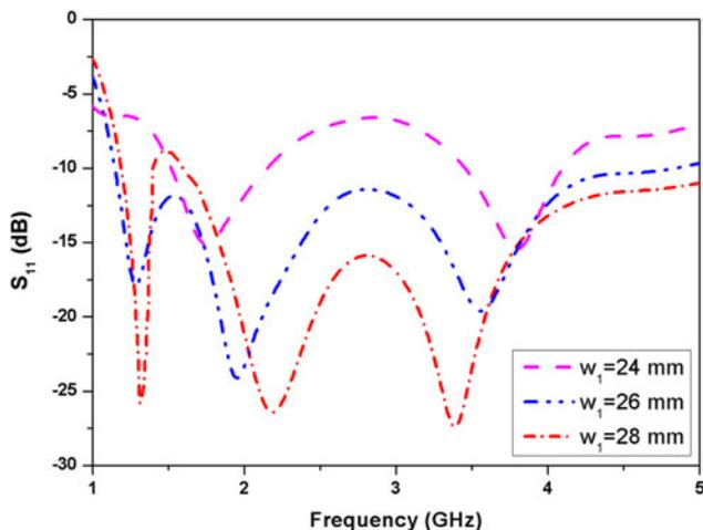
Fig. 9. Simulated  $S_{11}$  with different values of  $w_1$ .
