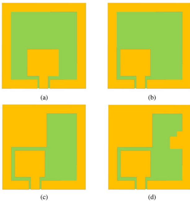
**Fig. 2.** Evolution steps of the proposed antenna: (a) Ant. 1, (b) Ant. 2, (c) Ant. 3, (d) Ant. 4.
