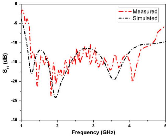
Fig. 4. Simulated and measured  $S_{11}$  of the proposed antenna.
