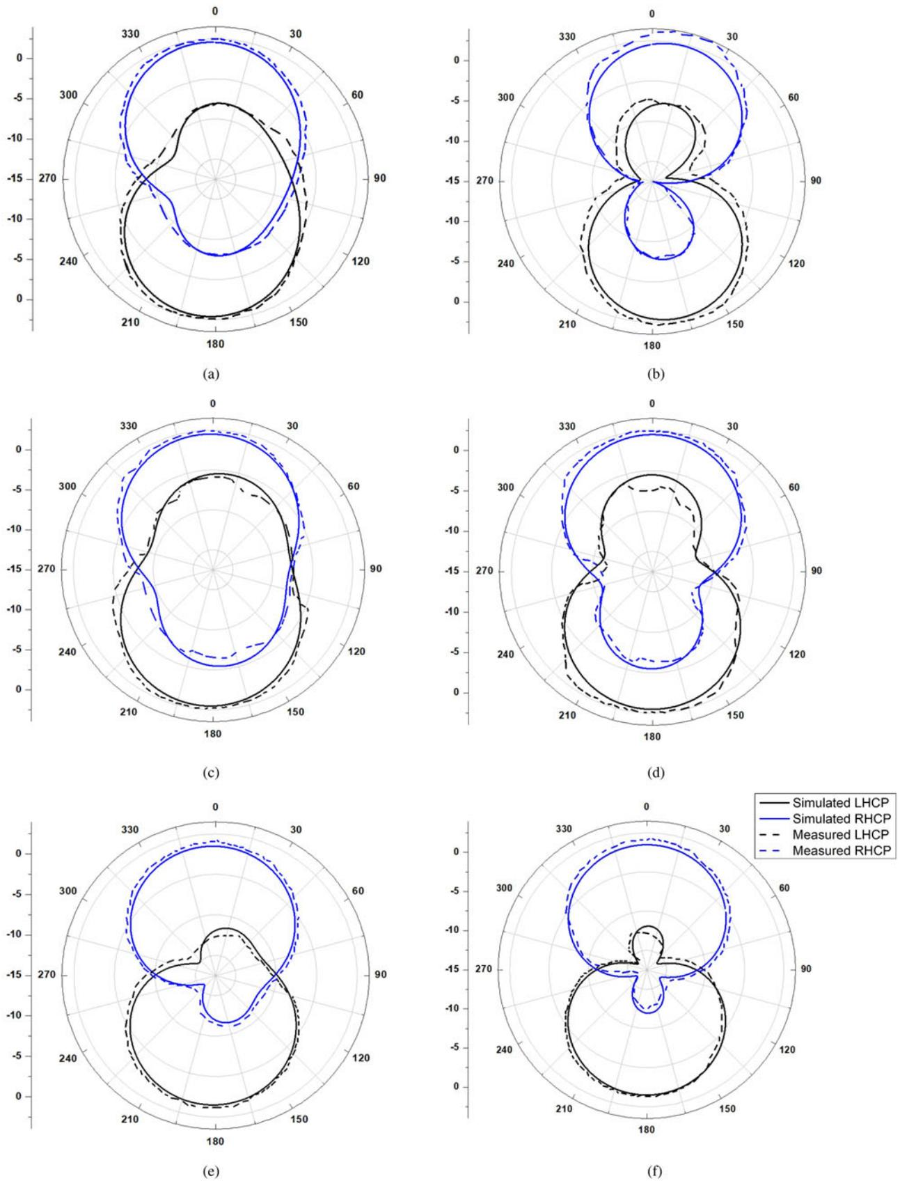
**Fig. 8.** Radiation pattern of the proposed antenna: (a) 1.17 GHz, XZ-plane; (b) 1.17 GHz, YZ-plane; (c) 1.22 GHz, XZ-plane; (d) 1.22 GHz, YZ-plane; (e) 1.58 GHz, XZ-plane; (f) 1.58 GHz, YZ-plane.
