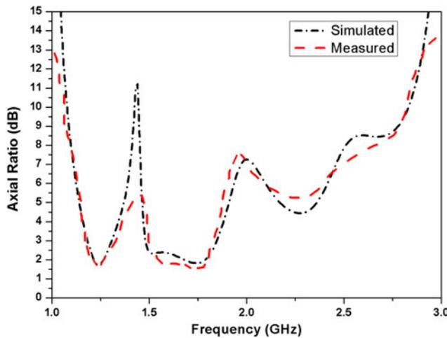
Fig. 5. Simulated and measured axial ratio of the proposed antenna.
