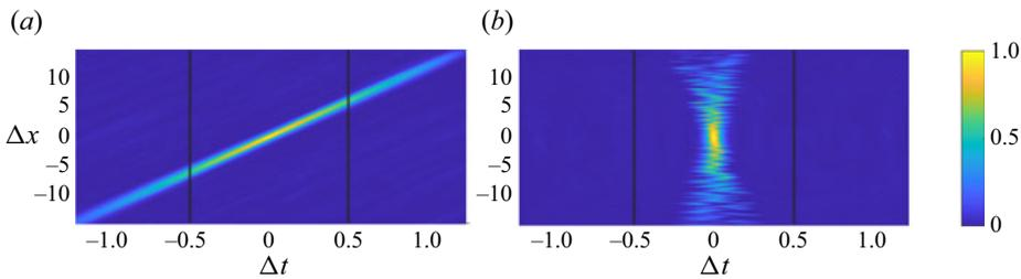
Figure 10. Space–time cross-correlation with respect to the point  $x_p = 15$  for case 2 ( $U = 12, A = 1$ ). Vertical lines represent the bounds of a window of size  $N_{FFT} = 100$ . Other cases display similar features. (a) No shift; (b) random  $U_{shift}(x) \in [0.8U, 1.2U]$ .
