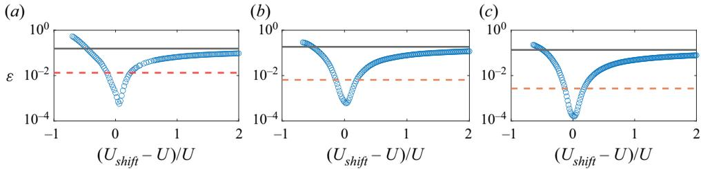
Figure 9. Estimation error  $\varepsilon$  of mode 1, at frequency  $\omega = 2\pi$ , number of snapshots  $N_{FFT} = 100$  and entire time series, as a function of the shifting velocity  $U_{shift}$ . Legend: (—) standard SPOD; (—, red) random  $U_{shift}(x) \in [0.8U, 1.2U]$  shifted SPOD; (o, blue) constant  $U_{shift}$  shifted SPOD. (a) Case 1; (b) case 2; (c) case 3.
