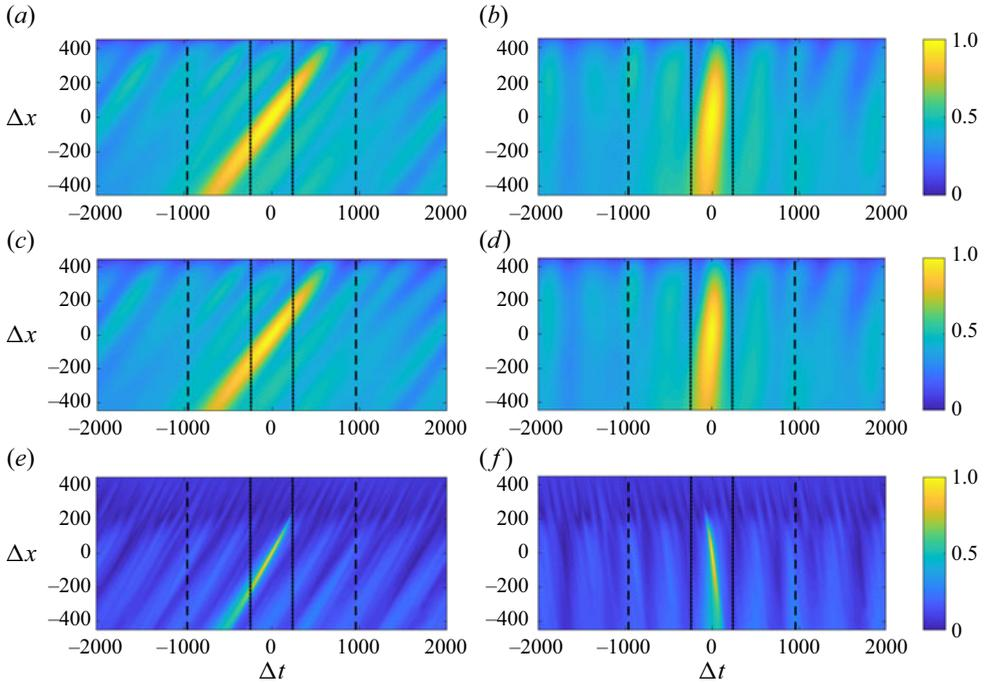
Figure 14. Space–time cross-correlation for  $\beta = 0.377$  of the  $u$  velocity component at different distances from the wall. Results are shown for (a,b)  $y = 0.01$ ; (c,d)  $y = 1$ ; (e,f)  $y = 6$ . (a,c,d) Non-shifted field. (b,d,f) Shifted field. Dashed line:  $N_{FFT} = 192$ ; dotted line:  $N_{FFT} = 48$ .
