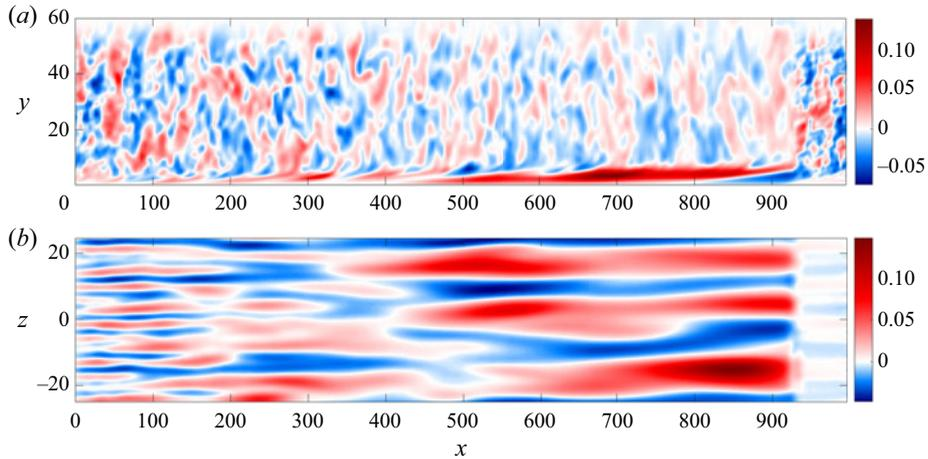
Figure 13. Snapshot of the LES, where elongated structures can be observed inside the boundary layer. Colours represent the streamwise velocity component. (a) Slice at  $z = 0$ . (b) Slice at  $y = 0.8$ . The fringe zone is visible after  $x = 900$ .
