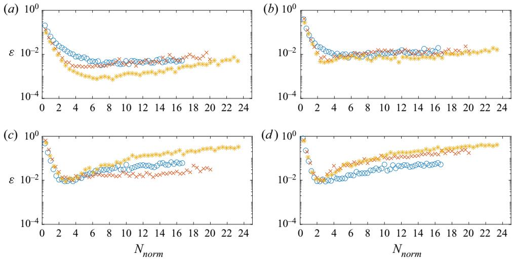
Figure 2. Spectral POD estimation error  $\varepsilon$  at frequency  $\omega = 2\pi$ , plotted against the normalised window length  $N_{norm}$ . Legend: ( $\circ$ , blue) case 1; ( $\times$ , red) case 2; ( $*$ , orange) case 3. (a) Mode 1; (b) mode 2; (c) mode 3; (d) mode 4.
