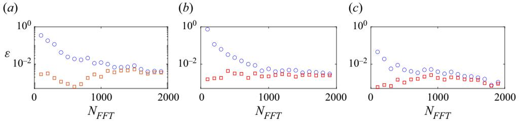
Figure 7. Estimation error  $\varepsilon$  of mode 1, at frequency  $\omega = 2\pi$  and number of blocks  $N_b = 100$ , as a function of the window size  $N_{FFT}$ . Legend: ( $\circ$ , blue) standard SPOD; ( $\square$ , red) shifted SPOD. (a) Case 1; (b) case 2; (c) case 3.
