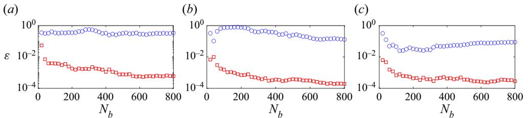
Figure 8. Estimation error  $\varepsilon$  of mode 1, at frequency  $\omega = 2\pi$  and number of snapshots  $N_{FFT} = 100$ , as a function of the number of blocks  $N_b$ . Legend: ( $\circ$ , blue) standard SPOD; ( $\square$ , red) shifted SPOD. (a) Case 1; (b) case 2; (c) case 3.
