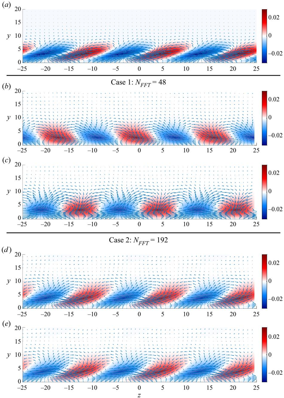
Figure 18. Section  $x = 700$  of the reconstructed modes. Legend: (colours)  $u$  velocity component; ( $\rightarrow$ ) perpendicular velocity component. (a) Resolvent response. (b,d) Standard SPOD. (c,e) Shifted SPOD.
