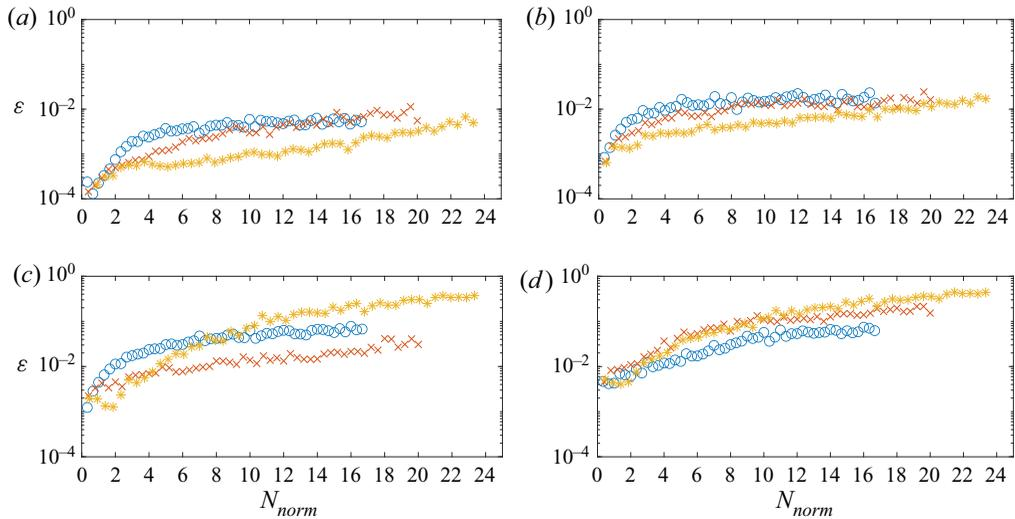
Figure 5. Shifted SPOD estimation error  $\varepsilon$  at frequency  $\omega = 2\pi$ , plotted as a function as  $N_{norm}$ . Legend: ( $\circ$ , blue) case 1; ( $\times$ , red) case 2; ( $*$ , orange) case 3. (a) Mode 1; (b) mode 2; (c) mode 3; (d) mode 4.
