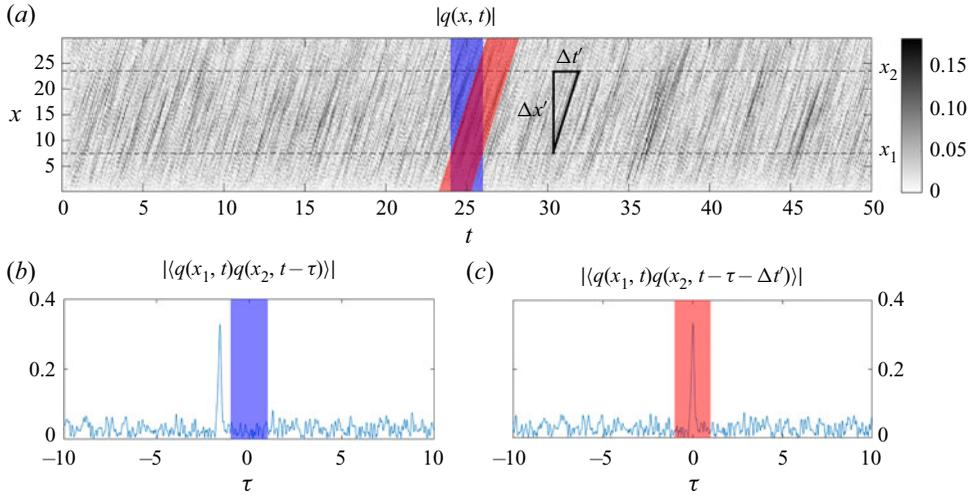
Figure 1. Diagram illustrating the effect of the temporal shift on the model system presented in § 5.1. In standard conditions, the cross-correlation peak lies outside the chosen time window. The application of the expected time lag between signals in positions  $x_1$  and  $x_2$  maintains the peak inside the same time window. The operator  $\langle \cdot \rangle$  denotes the expected value.
