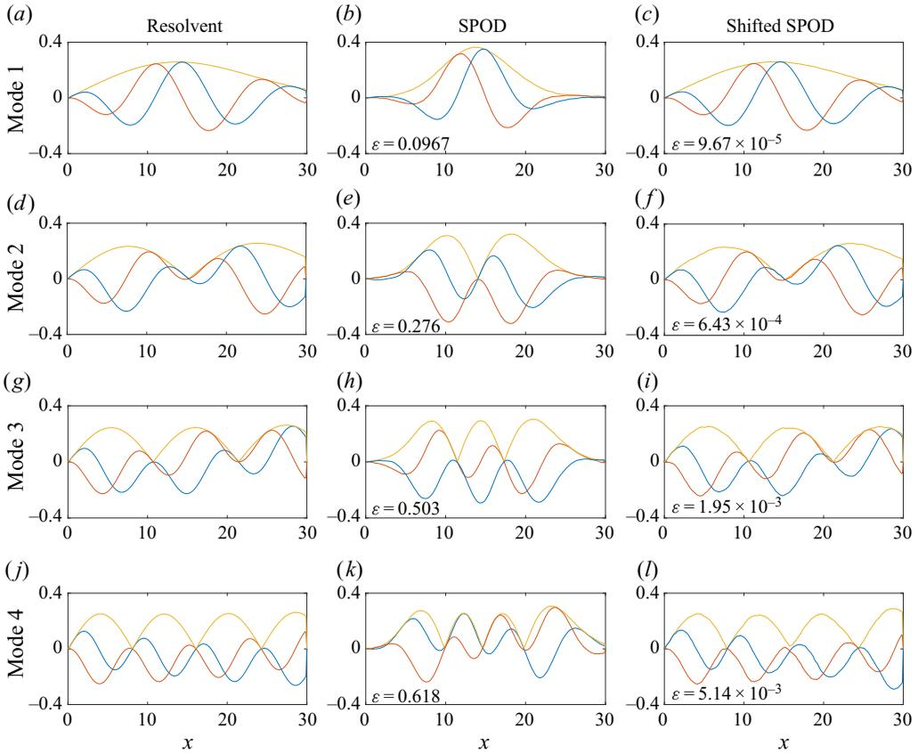
Figure 6. Comparison between resolvent, SPOD and shifted SPOD modes, at frequency  $\omega = 2\pi$ , for case 3. All SPOD modes were computed with  $N_{FFT} = 100$  and  $N_{norm} \approx 0.5$ . Other cases display similar features. Legend: (orange) absolute value; (blue) real part; (red) imaginary part.
