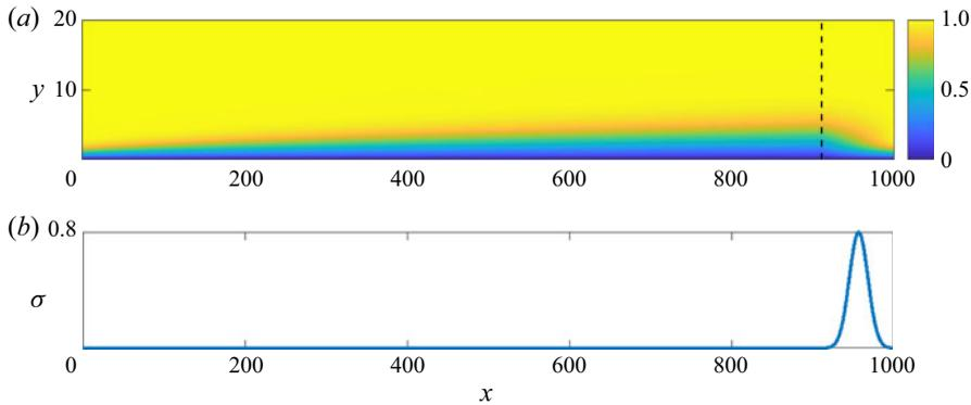
Figure 16. (a) Blasius mean velocity field ( $U$  component). The dashed line indicates the beginning of the fringe region. (b) Damping factor. The maximum of  $\sigma$  matches the value used in the LES.
