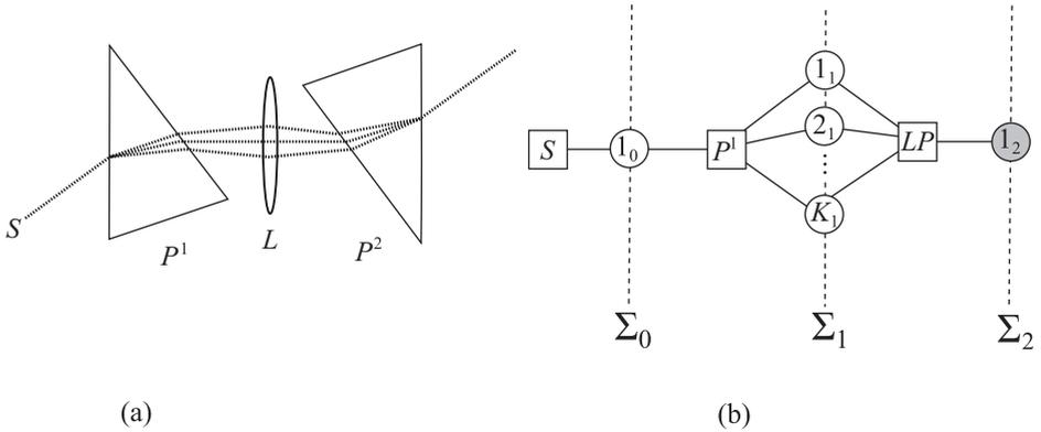
Figure 11.4. (a) Newton used lens  $L$  and prism  $P^2$  to recombine the spectrum from prism  $P^1$  back into a beam of white light. (b) In the QDN schematic of the same process, the lens and second prism constitute module  $LP$ .
