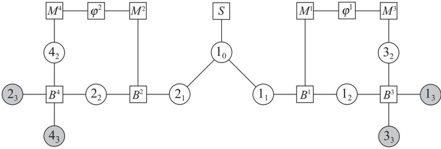
Figure 20.1. FRANSON-1: the Franson experiment for  $\Delta T < \tau_2 \ll \tau_1$ .  $S$  is the photon pair source, the  $B^i$  are beam splitters, the  $M^i$  are mirrors, and the  $\phi^i$  are phase changers.
