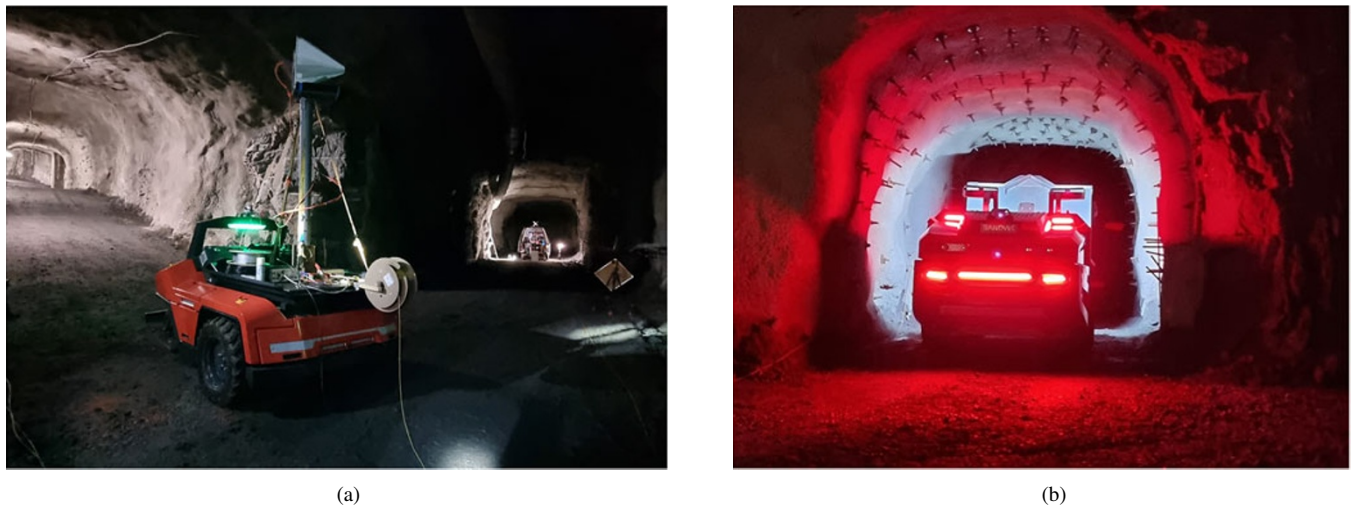
Figure 3. Vehicles utilized in the measurement campaigns. (a) FR1 NLOS measurement at crossroad 1. In middle, the TX antenna on ECV and the van with the RX antenna is at end of the main tunnel. (b) FR1 NLOS measurement: Loader blocks a narrow side tunnel.
